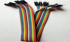
Fig. 5. Jumper Wires
