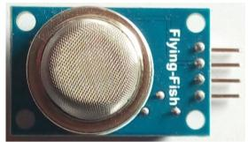
Fig. 3. MQ135 CO<sub>2</sub> Sensor
